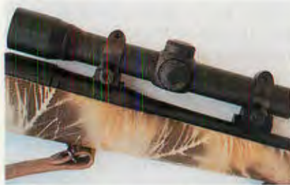
Burriss 2.75X fixed power, long-eye-relief scope with standard duplex reticle pattern is attached to the Gunsite Scout Rifle by integral barrel scope mounts and Warne in-line rings.
